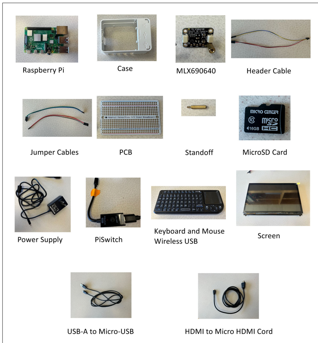
Figure 1 Component organization. All necessary components for the thermal camera assembly are laid out and identified, including the Raspberry Pi, case, thermal camera, cables, PCB, and peripherals.
