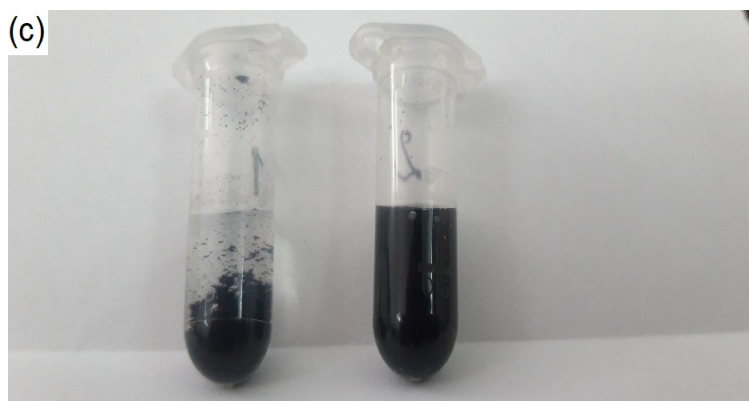
Figure 3. SEM morphological details of CNTs as received from the manufacturer, before (a) and after (b) loading with the mixture CHX/AgNPs (High magnification, 100,000×); (c) photographic image of colloidal CNTs in distilled water (left) compared to colloidal mixture CHX/AgNPs (right).
