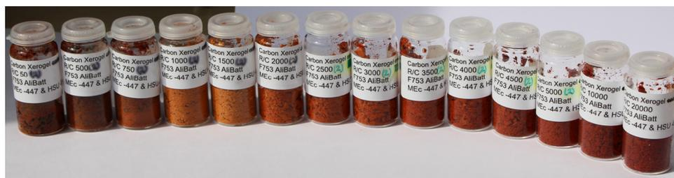
**Figure 1.** As-prepared resorcinol-formaldehyde resins after drying step from high catalyst concentration ( $R/C = 50$ ) on the left side to low concentration ( $R/C = 20,000$ ) on the right side.
