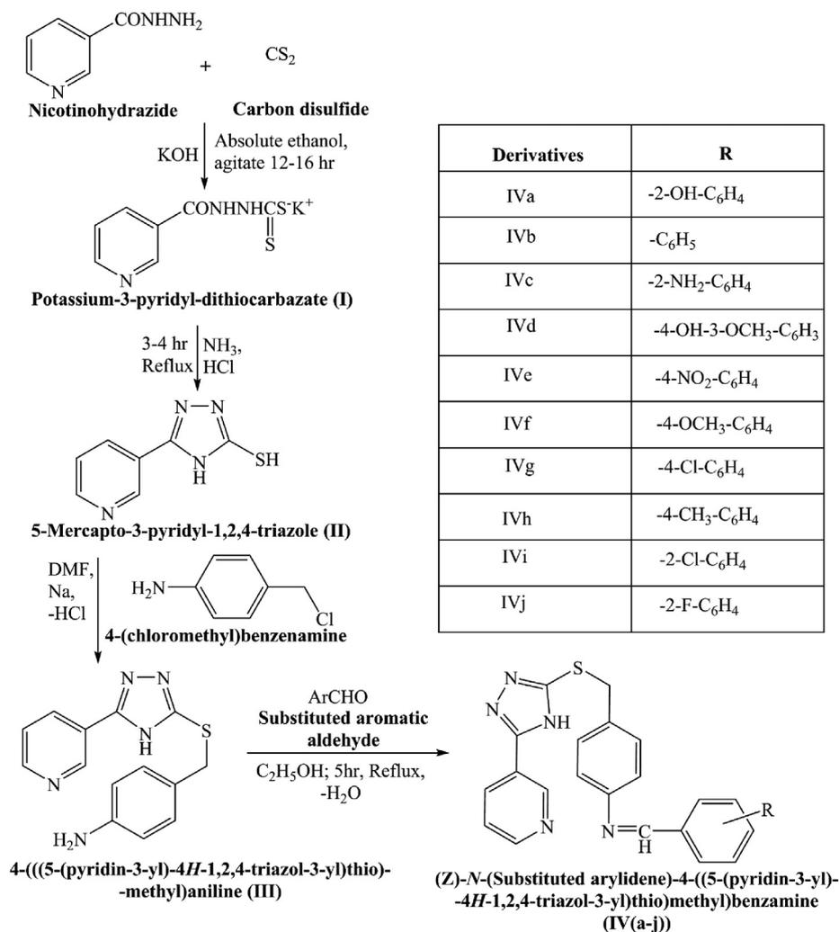
Fig. 1. Scheme for the preparation of various 1, 2, 4-triazole pyridine hybrids Schiff base.
