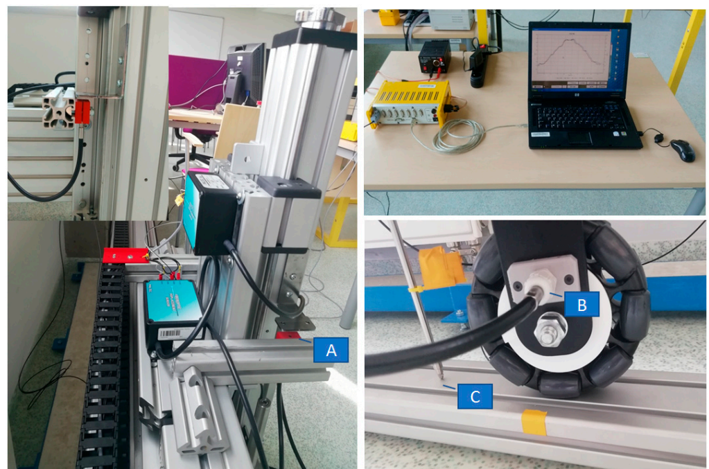
Figure 6. Position of the measuring instrumentation. (A) optical sensors, (B) optical sensors, (C) LVDT displacement sensor.
