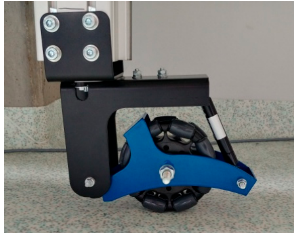
Figure 10. View of the vertical upright with the installed suspension system.
