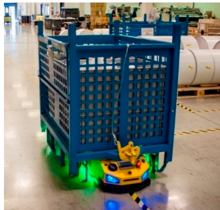
Figure 1. Tractor-type AGV Pull500 manufactured by Etisoft Smart Solutions Sp. z o.o.
