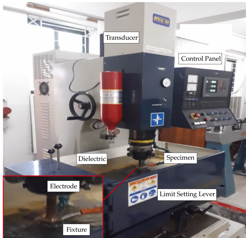
Figure 2. Experimental setup for EDM.
