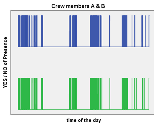
Fig 4. Comparison of two sensor's data. Presence–absence detections between two sensors (crewmembers A and B) over one mission day registrations.
