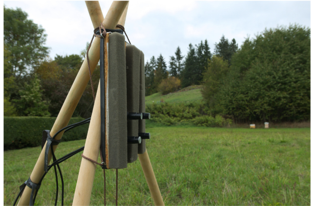
Figure 1. Setup used for testing microphone attachments outdoors. The microphones were approximately 1 m above the ground and parallel to each other.
