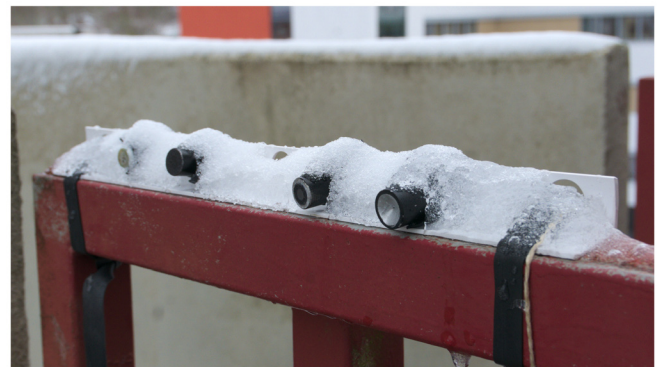
Figure 2. Different microphone prototypes exposed to outdoor conditions during winter 2021 in Germany.
