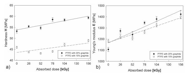
**Figure 6.** Impact of electron beam irradiation on changes in microhardness H (**a**) and modulus of elasticity E (**b**) of PTFE-graphite composites.
