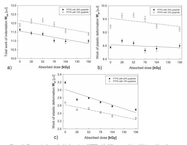
**Figure 7.** Changes in the work of indentation of PTFE with different graphite additions subjected to an absorbed dose of electron beam irradiation: the total work of indentation— $W_{tot}$  (a), the work of plastic deformation— $W_{pl}$  (b), and the work of elastic recovery  $W_{el}$  (c).
