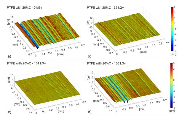
**Figure 11.** Stereometric structure of the friction surface of PTFE with a 20% graphite addition in its initial state 0 kGy (**a**) and after absorbing a dose of 52 kGy (**b**), 104 kGy (**c**), 156 kGy (**d**).
