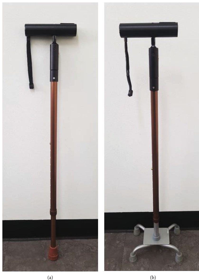
FIGURE 2: Types of cane-supported gait using a weight-support feedback cane (WSFC). WSFC can be used in a mono cane (a) and in a quadripod cane (b) by switching the cane's legs.
