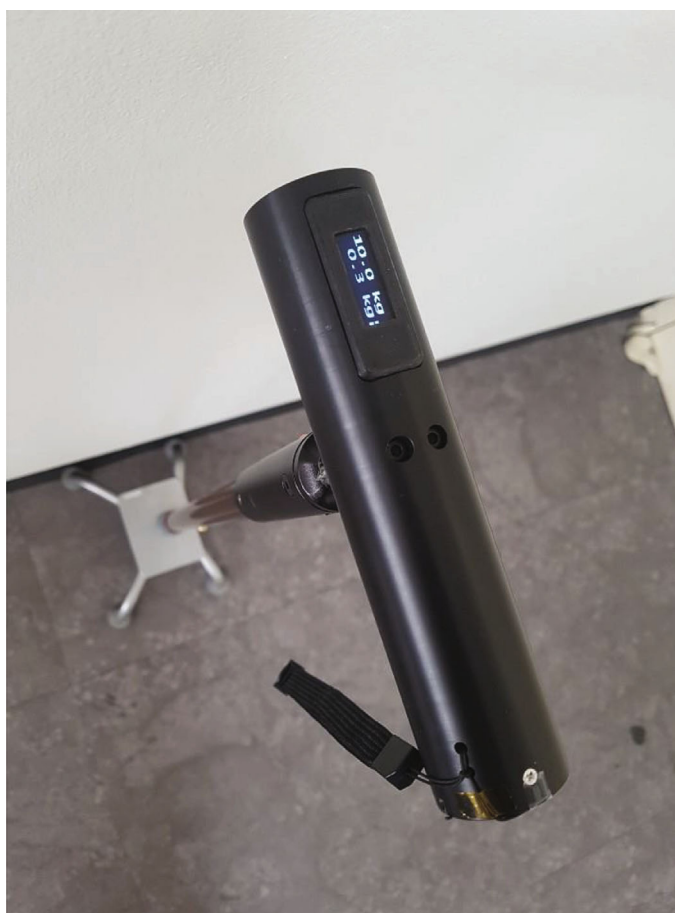
FIGURE 1: A weight-support feedback cane (WSFC). The WSFC measures cane dependence (degree of weight support loaded on the cane (kg)) during walking. Measurement of the degree of weight support occurs through a load cell located inside the bottom of the cane handle. The degree of weight support is displayed in real time on the cane handle’s top display.
