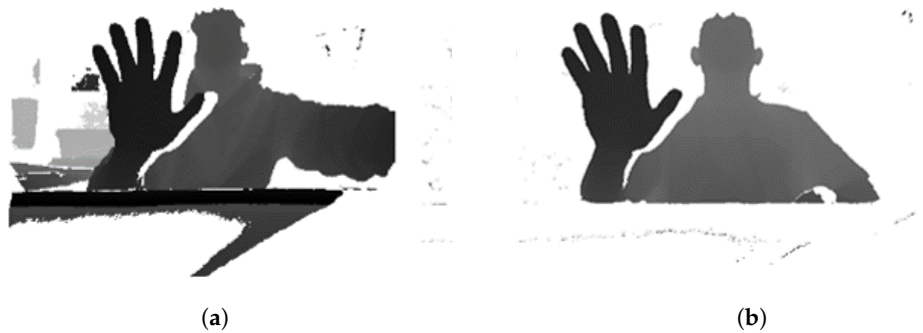
Figure 9. The experimental result before (a) and after (b) of applying the background subtraction.
