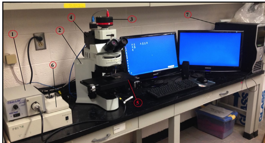
FIGURE 1 CytoViva® Hyperspectral Imaging Microscope System. 1: Halogen light source; 2: optical microscope; 3: optical camera; 4: VNIR spectrophotometer; 5: motorized stage; 6: controller for stage; and 7: computer
