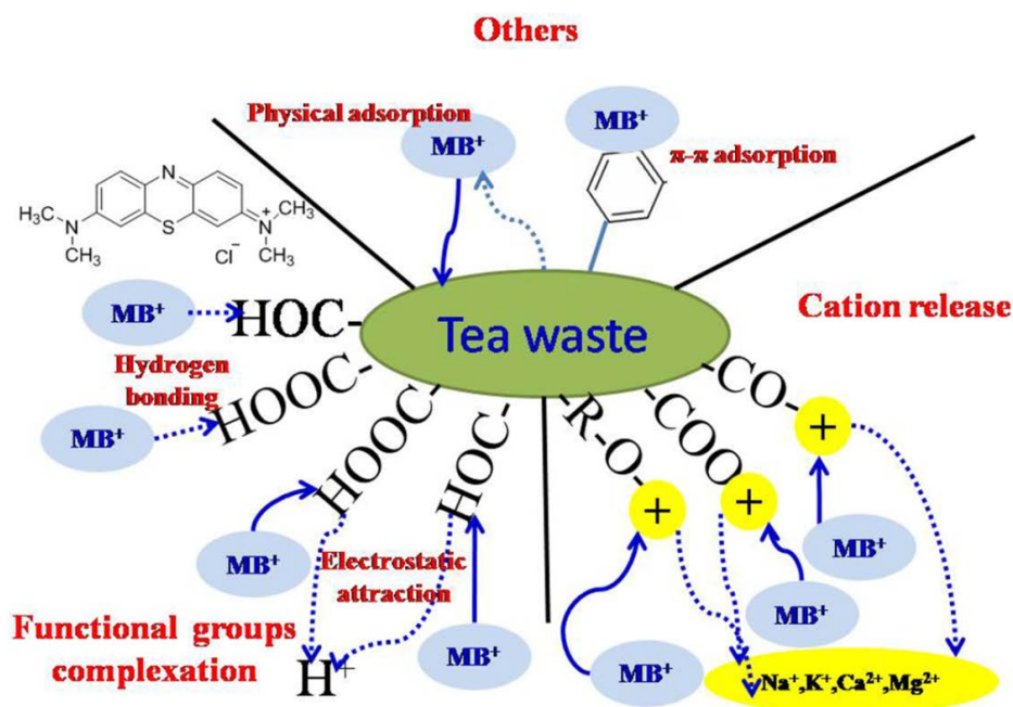
Figure 6. Mechanism diagram between tea waste and methylene blue.
