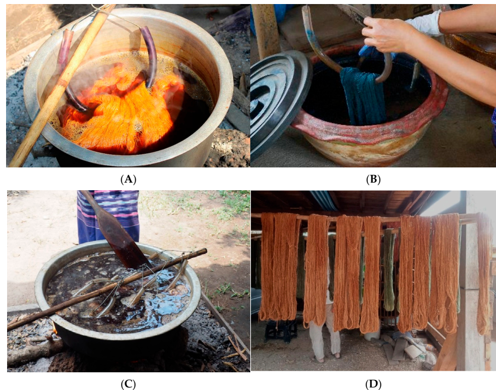
Figure 6. The dyeing process of yarn (A,B) The yarns were immersed in the prepared dye extraction solution; (C) Utilize a spatula to press the yarn into the dye solution; (D) The dyed yarns were suspended on strings in the shade to naturally dry.
