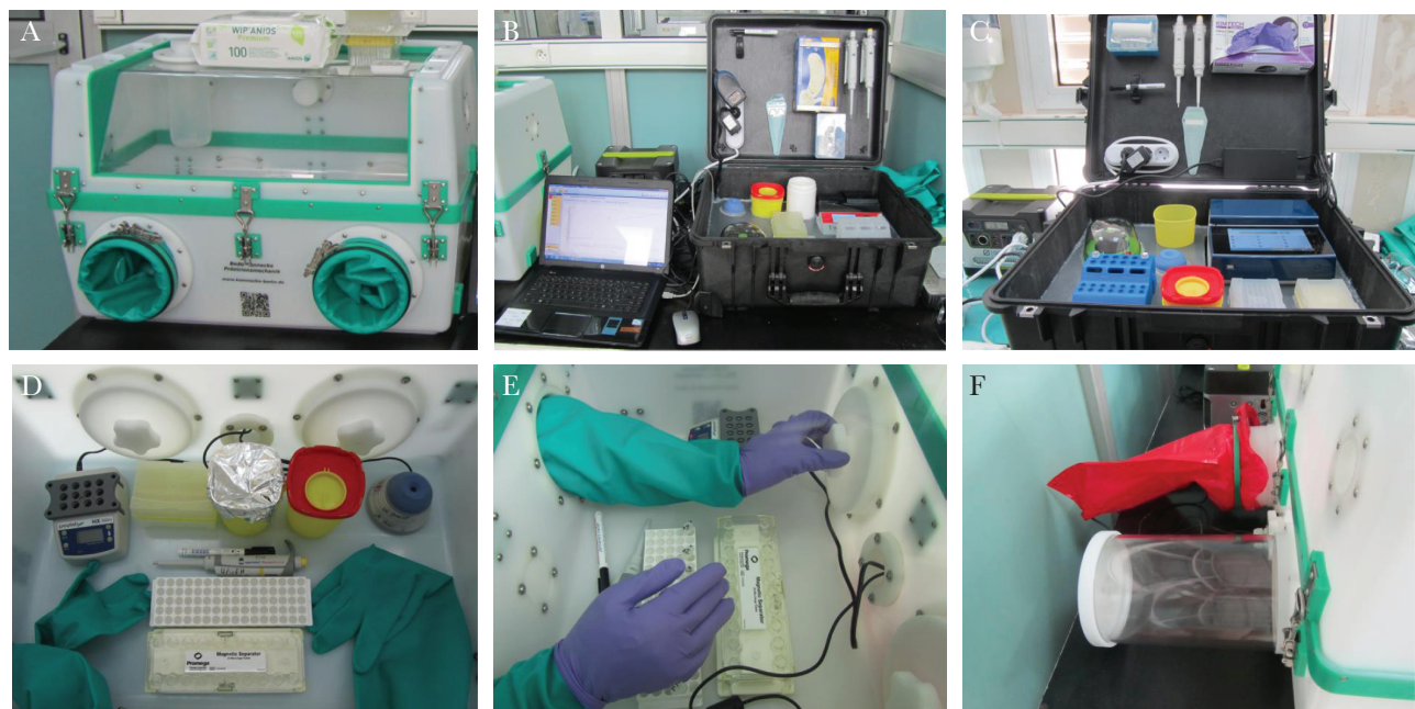
Figure 3. Mobile laboratory (ML4) pipetting. (A) Extraction in glovebox. (B) ML4a Real-time recombinase polymerase amplification (RT-RPA) in development of a suitcase laboratory (DiaS). (C) The ML4b and 2 RT-RPA in DiaS (Tubescanner II, no laptop). (D) Details of setup for extraction. (E) Opening of internal door of export lock. (F) Export lock and waste bag attachment.
