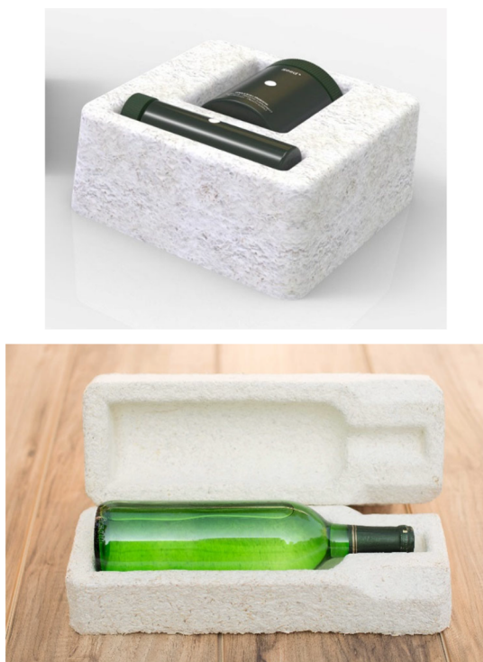
Figure 10. Mycelium composite foams used to package consumer products. Reprinted by permission from Ecovative Design LLC, Copyright 2019.
