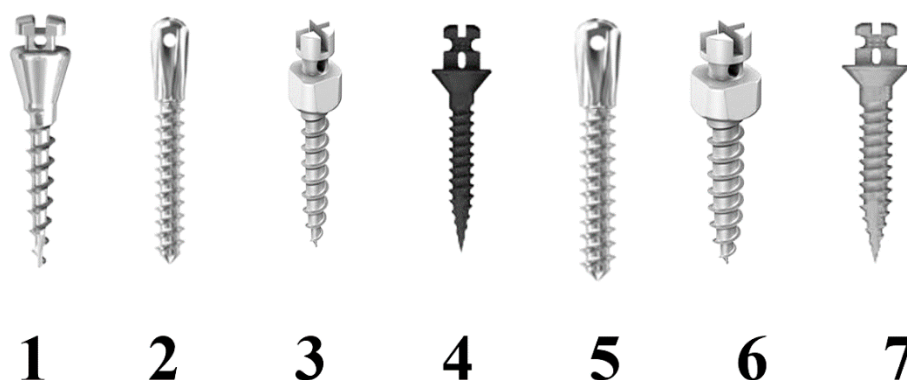
Figure 1. Miniscrews with different diameters tested in the present investigation. 1: 1.5 mm HDC—2: 1.5 mm Leone—3: 1.5 mm Orteam—4: 1.5 mm Kristal—5: 2.0 mm Leone—6: 2.0 mm Orteam—7: 2.0 mm Kristal.
