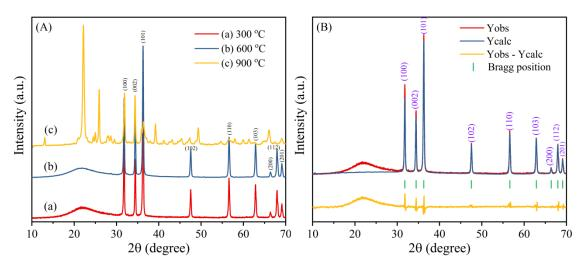
**Figure 2.** (**A**) XRD patterns of ZS1 annealed at various temperatures and (**B**) Rietveld Refined XRD pattern of ZS1<sub>300</sub> nanocomposite.
