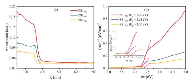
Figure 5. (a) UV plots (b) Tauc's plot of ZS1300, ZS1600 and ZS1900.
