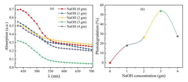
**Figure 10.** Effect of NaOH on catalyst; (a) UV–visible spectra for different concentrations of NaOH and (b) photo-degradation efficiency w.r.t. concentration NaOH.
