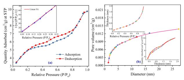
**Figure 6.** BET isotherm of ZS1<sub>300</sub> (**a**) adsorption and desorption curve and (**b**) pore size distribution, the thickness of deposited layer (inset) & adsorption quantity versus size of the pore (inset).
