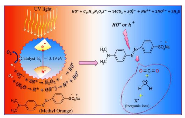
Scheme 2. Schematic illustration of the photocatalytic mechanism of ZnO.SiO<sub>2</sub> photocatalyst for degradation of MO.
