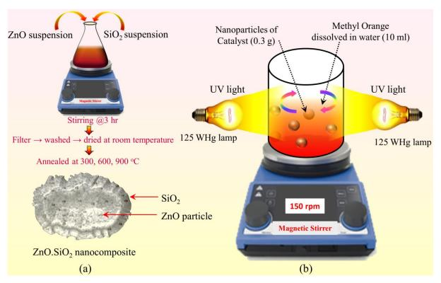
**Scheme 1.** Schematic diagram of ( $\mathbf{a}$ ) preparation of SiO<sub>2</sub>.ZnO nanoparticles with the expected morphology (ZnO nanoparticles embedded into SiO<sub>2</sub> porous structure) and, ( $\mathbf{b}$ ) photocatalytic activity set-up.
