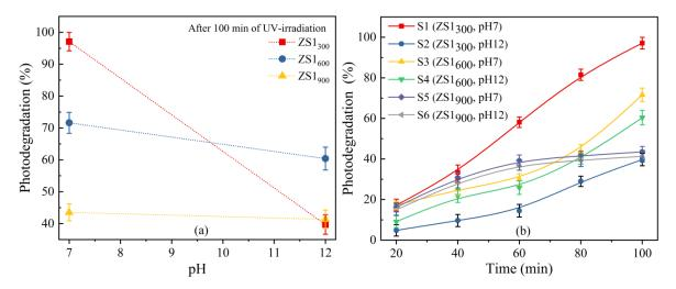
Figure 8. Effect of (a) irradiation time and (b) pH on photodegradation rate (%) of methyl orange (UV irradiation =  $(2 \times 125)$  W).
