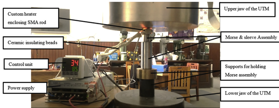
Figure 6. Experimental setup to simulate the implementation of AD during the extraction of a Morse rod from its sleeve.
