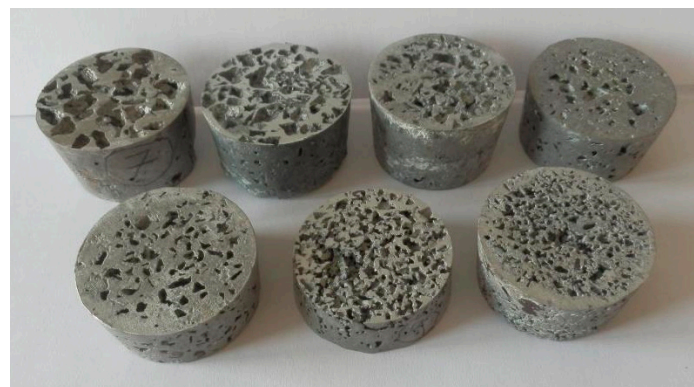
Figure 6. View of manufactured samples of aluminium porous material, AlSi12 alloy, in the shape of a truncated cone (the samples are not sorted by number).
