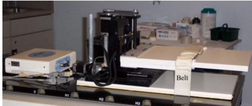
Fig. 1. Motion platform used to simulate breathing patterns with the motion-monitoring system. Adjustable belt is placed around the platform to monitor the AP motion direction.
