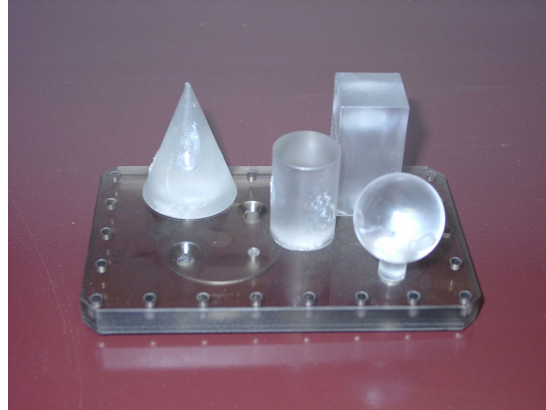
Fig. 3. Radiosurgery QA phantom including conical, cylindrical, rectangular, and spherical test objects. This phantom was used for gating method comparisons.
