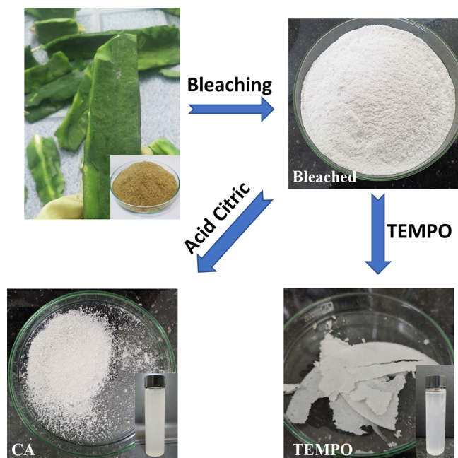
Figure 1. Procedures to extract nanocellulose from dragon fruit foliage by different approaches including (2,2,6,6-tetramethylpiperidin-1-yl)oxyl (TEMPO) and citric acid.
