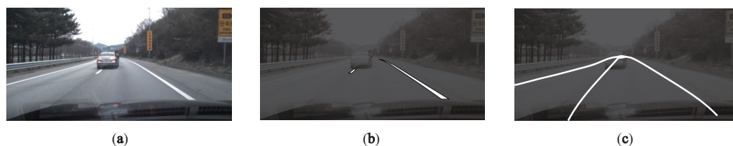
Figure 1. Example for lane detection output difference according to approaches. (a) Original Image, (b) Feature-based Lane Detection, (c) Learning-based Lane Detection.
