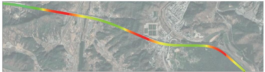
Figure 18. Scenario 4: GNSS signal outage in tunnels. Green denotes low dilution of precision, and red denotes high.
