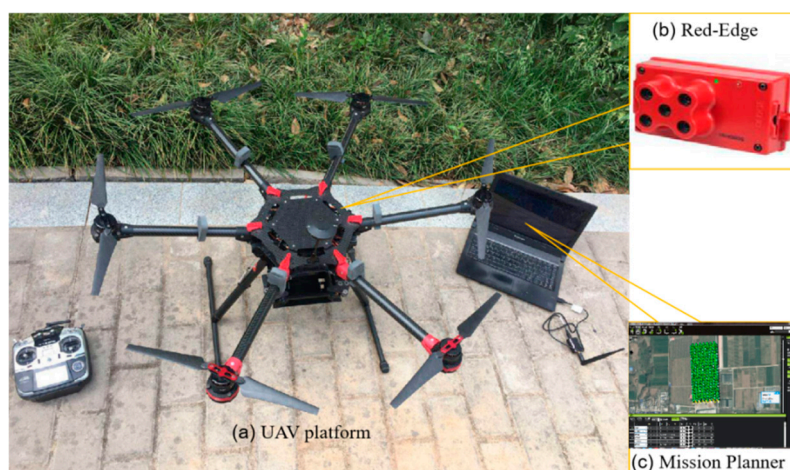
Figure 2. The main elements of the UAV multispectral remote sensing system. (a) UAV platform (b) RedEdge multispectral camera, and (c) the software, Mission Planner.
