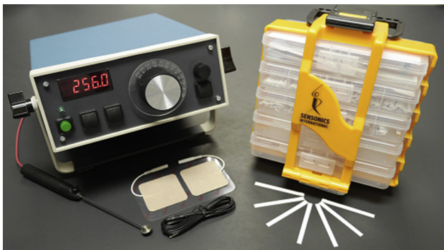
Fig. 8 Left: A modern electrogustometer and its electrodes. This device can apply a wide range of perithreshold currents with the electrode on the tongue being either the anode (standard confirmation) or cathode. Right: A modern clinical taste testing system employing plastic disposable tabs whose ends are embedded with tastants. Photograph courtesy of Sensonics International, Haddon Heights, New Jersey USA. Copyright © 2017 Sensonics International.
