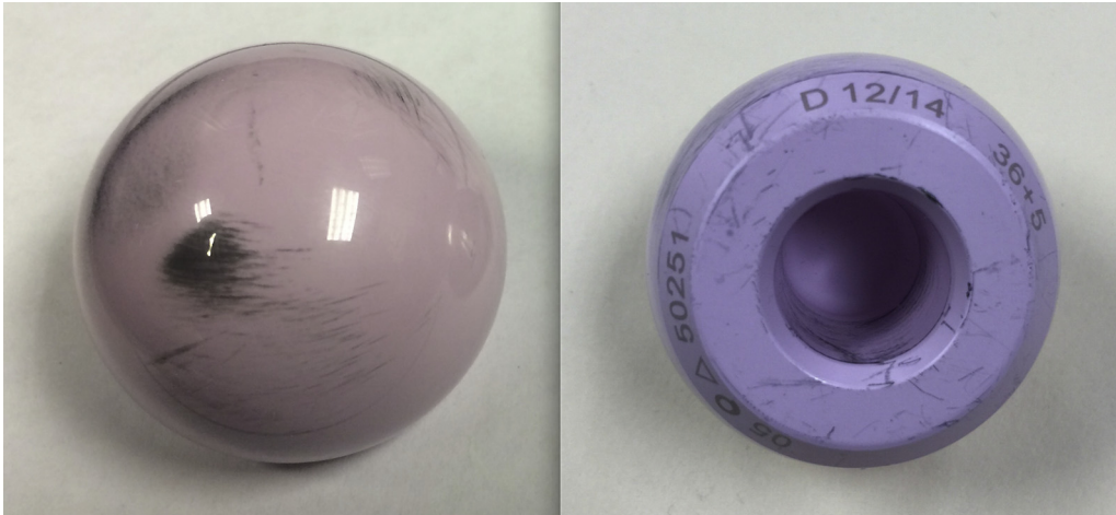
Figure 3. Photographs of explanted Biolox (CeramTech, Plochingen, Germany) Delta ceramic femoral head. There is evidence of metal transfer onto the ceramic femoral head.
