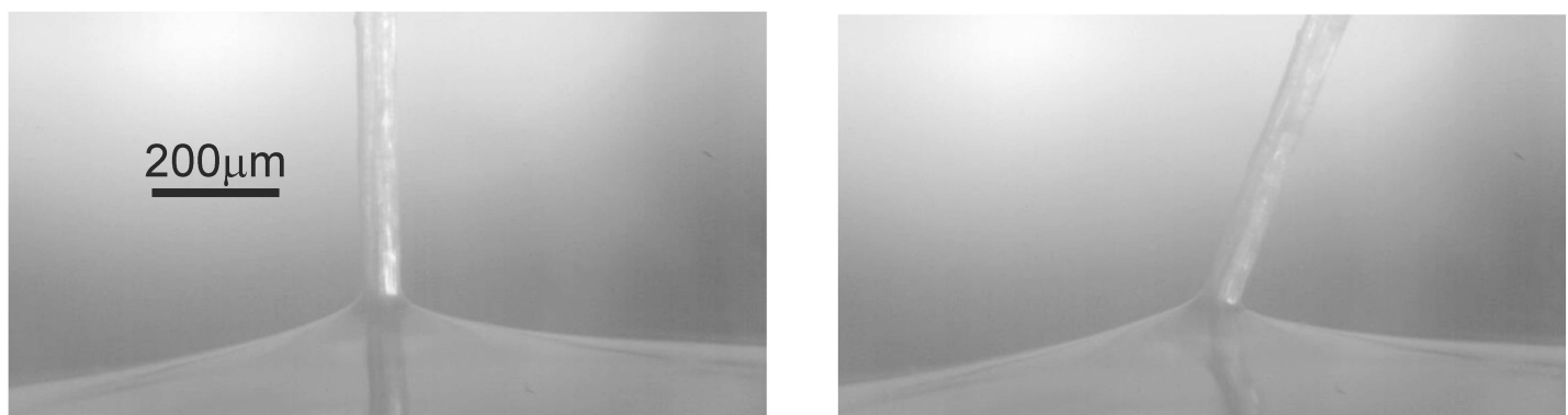
Fig 2. Foot fixation of the stem. The stem of the pappus sensor is fixated at the bottom wall in a thin silicone rubber membrane. Sensor at rest (left) and under strong wind load (right). Note that the stem keeps its straight shape under load.
