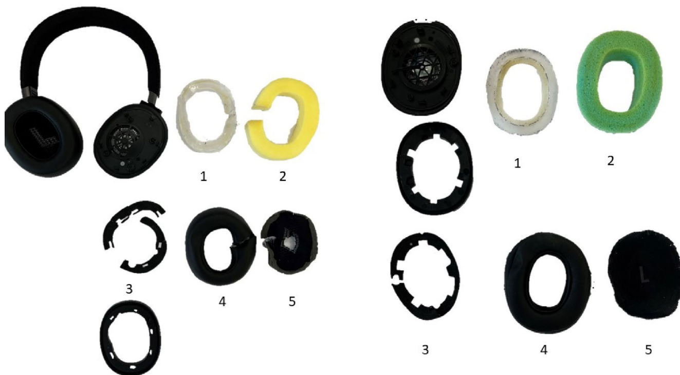
FIGURE 4 | Different parts of the culprit headphones of the Patient 1 (left side) and 2 (right side), that were analysed using UPLC-MS/MS.
