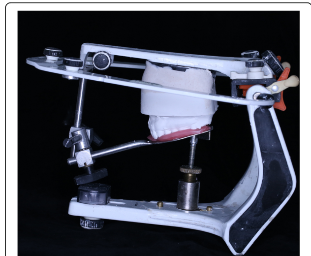
Fig. 2 Transfer of the face-bow record to the semi-adjustable articulator to allow for accurate mandibular cast mounting
