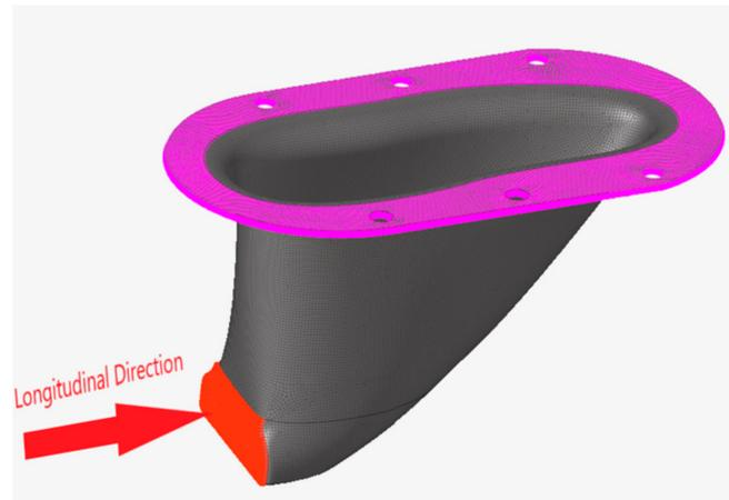
**Figure 4.** Boundary constraint location at the top of the structure (pink) and load application location on the front, bottom of the structure (red) and the longitudinal load application direction.
