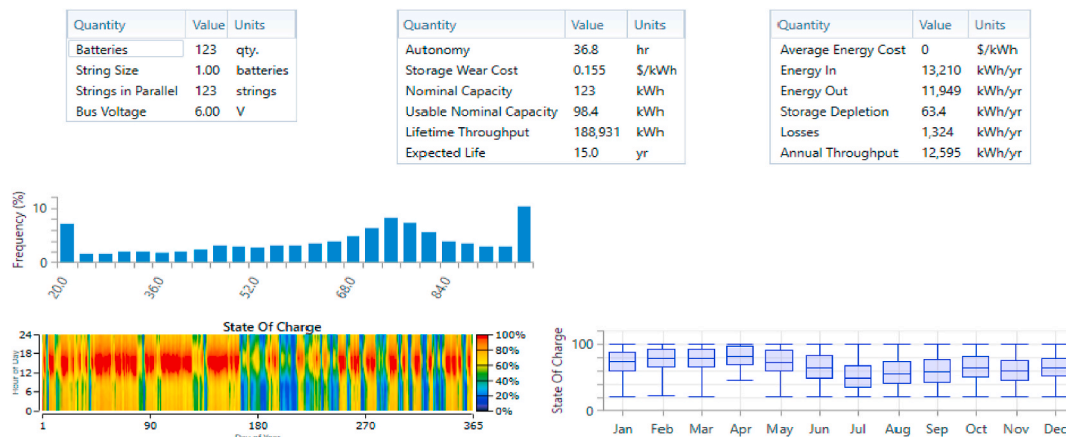
Fig. 5. Battery specifications of the system.
