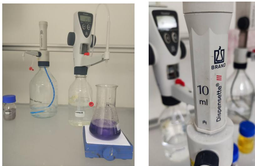
**Figure 5.** Pictures of titration equipment, EDTA method setup.
