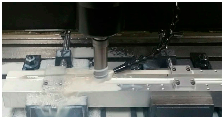
Figure 3. Milling of the preform on a customized milling stage with Standard Series 10 Rotary Knee mill from Sonic-Mill.
