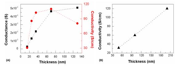
**Figure 3.** (A) Conductance (black squared symbols) and conductivity (red circles) as a function of the device channel thickness for long-lasting thermal annealing (LTA) processing; (B) Conductivity versus channel thickness for films processed under rapid thermal annealing (RTA) conditions.
