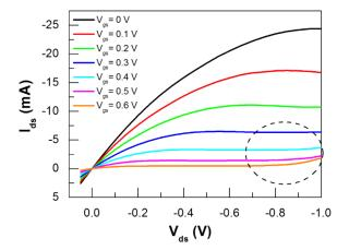
**Figure 2.** Output characteristics of an OECT with a 70-nm-thick PEDOT:PSS channel recorded by sweeping  $V_{\rm ds}$  between 0.05 V and -1 V at a scan rate of 50 mV/s and a constant gate bias ( $V_{\rm gs}$ ) fixed between 0 and 0.6 V, with  $V_{\rm gs}$  steps of 0.1 V. The dotted circle corresponds to the onset of the electrolysis of the aqueous sodium chloride electrolyte.
