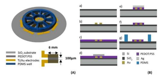
**Figure 1.** (A) Organic electrochemical transistor (OECT) layout. (B) Device fabrication process: (a)  $SiO_2$  substrate, (b) patterned electrical contacts, (c) poly(3,4-ethylenedioxythiophene):polystyrene sulfonate (PEDOT:PSS) film, (d) Ag layer, (e) excess of PEDOT:PSS removed by  $O_2$  plasma, (f) Ag removal by E6 wet etching, and (g) bonding of poly(dimethylsiloxane) (PDMS) well.
