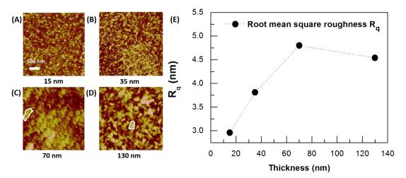
**Figure 5.** AFM micrographs for **(A)** 15-, **(B)** 35-, **(C)** 70-, and **(D)** 130-nm-thick PEDOT:PSS films (scale bar 500 nm; white circles indicate typical PEDOT domains); **(E)** saturated root mean square roughness  $(R_q)$  as a function of the device channel thickness.
