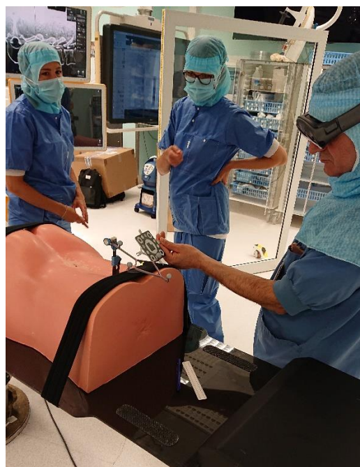
Figure 9. The surgeon calibrating the HMD to the navigation system using a hybrid marker.
