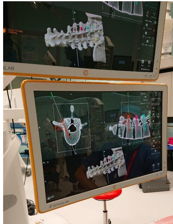
Figure 2. The screens of the navigation system present information corresponding to the surgeon's view in the HMD.
