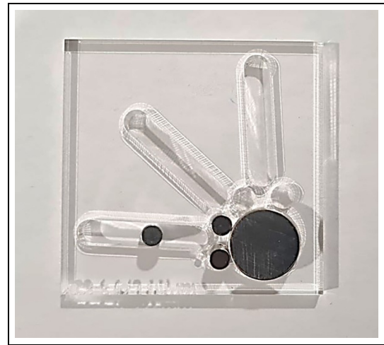
Figure 3. Example of pegboard. Printed 3D model with magnets inserted into the pegboard.
