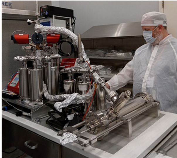
Fig. 14 Piercing tool integrated with the gas extraction manifold
