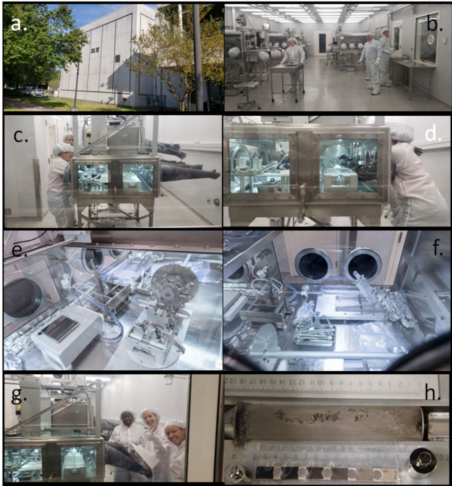
Fig. 30 (a) Building 31N, the home of JSC lunar sample curation facility. (b) Apollo lunar sample clean lab. (c and d) Glove box within the Apollo lunar sample clean lab used for the extrusion, dissection, sieving, and documentation of 73001 and 73002. (e and f) tools in the glove box that were used for extrusion and dissection of tools. (g) Successful extrusion of double drive tube 73002. (h) Extruded core 73002 prior to derinding and dissection
