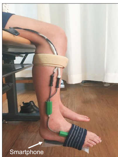
Figure 1. Attached smartphone and electrogoniometer.
