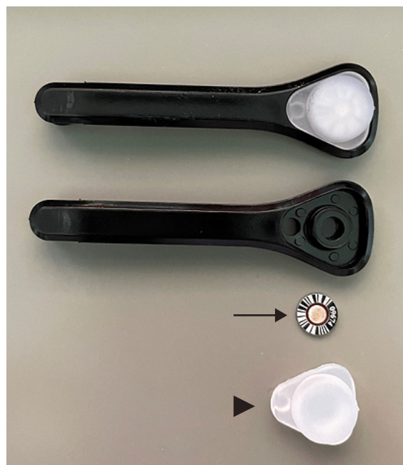
Figure 3. The detector is a thermoluminescent dosimeter (TLD, arrow) that uses {}^7\text{LiF:Mg,Ti} as the TLD element and is encapsulated in a 3-mm-thick polypropylene capsule (arrow head).
