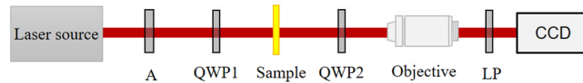
Figure 3. Schematic diagram of the experimental setup. A: attenuator; QWP: achromatic quarter-wave plate; LP: linear polarizer; CCD: charge-coupled device.
