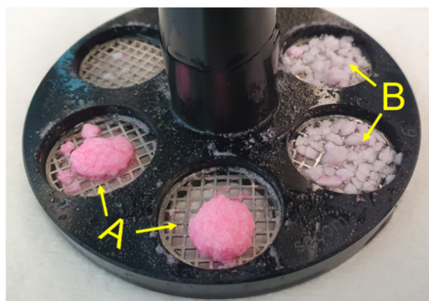
Figure 5. Tablet residues on the screen after a 30 min standard disintegration test (SDT) at modified average fluid velocity (9 mm/s). Coarse tablet residues visible for tablets containing 78% MCC and 20% Kollidon VA64 (A); finer tablet fragments visible for tablets containing 78% MCC and 20% Eudragit EPO (B). All tablets contained 2% PVPP as disintegrant and had a porosity of 0.2.
