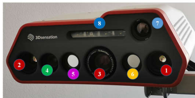
Figure 1. Multimodal 3D imaging system. 1/2: High-speed cameras at 850 nm, 3: High-speed GOes Before Optics (GOBO) projector at 850 nm, 4: Color camera, 5: NIR camera at 780 nm, 6: NIR camera at 940 nm, 7: Thermal camera, 8: Light emitting diode (LED) array at 780 and 940 nm.
