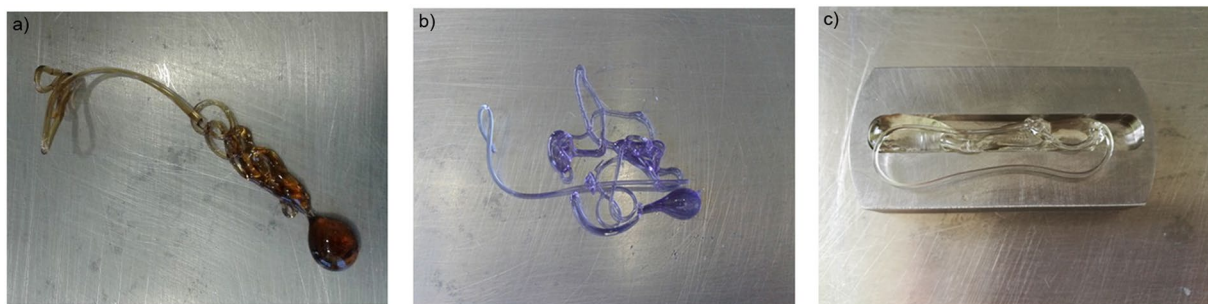
Figure 11. Poured glasses for the Matrix-Ce30 (a), Matrix-Nd30 (b) and Matrix-Eu30 (c) compositions.
