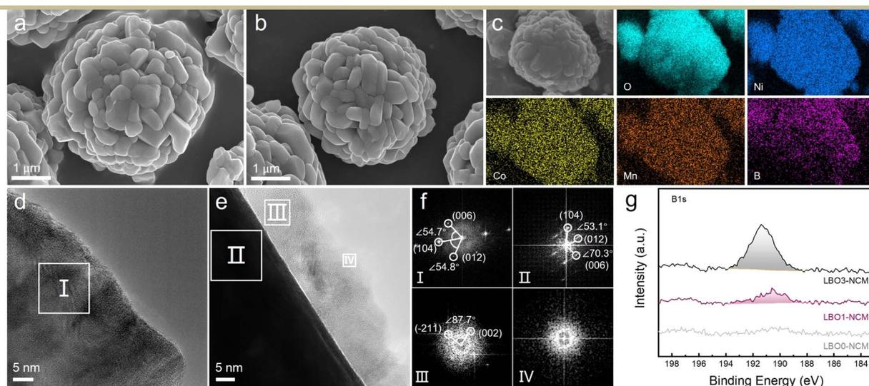
**Fig. 1** SEM images of (a) LBO0-NCM and (b) LBO1-NCM. (c) Elemental mapping images of LBO1-NCM. HRTEM images of (d) LBO0-NCM and (e) LBO1-NCM. (f) Corresponding FFT patterns of areas I, II, III, and IV. (g) XPS spectra of LBO0-NCM, LBO1-NCM, and LBO3-NCM.
