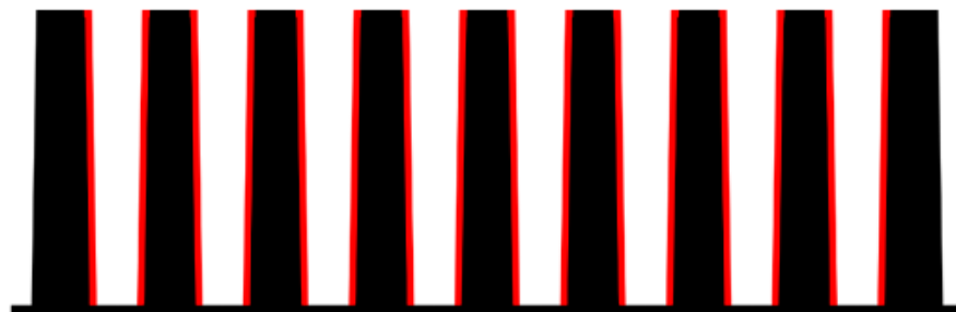
Figure 14. Fins' surfaces (red) whose radiative heat transfer coefficient needs to be adjusted due to their mutual radiation.
