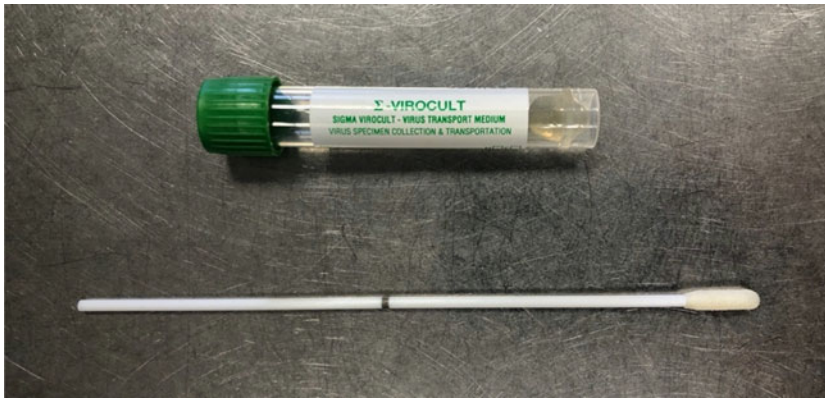
Fig. 2. Viral swab with breakpoint mechanism (black line on the swab shaft) and accompanying bottle containing virus transport medium.
