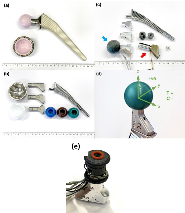
FIGURE 1. The stock implant (Corail Hip Systems, DePuy Synthes, Johnson&Johnson, Warsaw IN, USA) was used as the starting basis for the design of the instrumented prototypes. (a) The permanent implant and (b) the temporary (trial reduction) implant with various modular neck and head geometries. (c) The instrumented prototype with instrumented necks and a modified head. The blue arrow indicates the 3DOF prototype and the red arrow indicates the 1DOF prototype. (d) The coordinate system used in this report; tension (or compression from the negative side of the axis) is positive while compression is reported as negative. (e) The inside of the 3DOF implant with the head removed shows the radial and axial O-rings, sensor placement and wiring.
