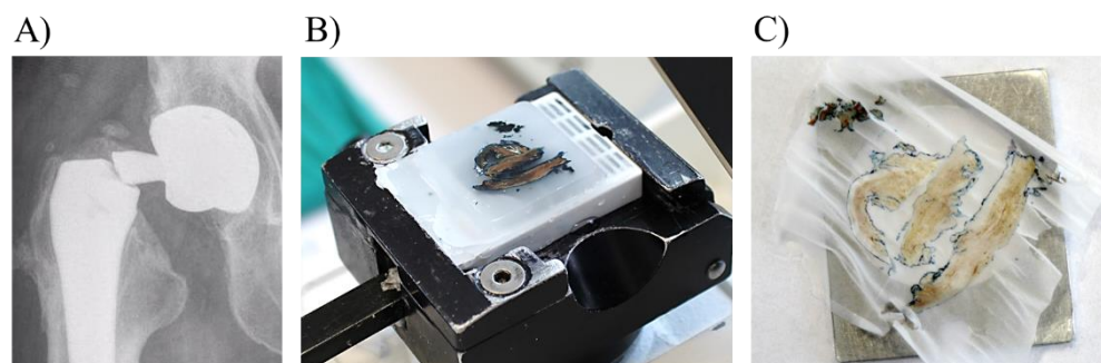
Figure 2. Collection and preparation of periprosthetic tissue slices for multimodal and multiscale analysis. (A) X-ray image from fractured modular neck (B) paraffin embedded periprosthetic tissue placed in the microtome (C) microtome sectioned tissue slice over the aluminium frame with mylar window.
