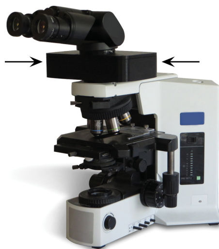
Fig. 1. Optical Module (arrows) installed on any existing light microscope. Copied with permission from: Siegel S, Regelman R, Maronpot RR, Rosenstock M, Nyska A (2017). New technologies: real time telepathology systems—novel cost-effective tools for real-time consultation and data sharing. Toxicologic Pathology 45(8): 1039–1042.
