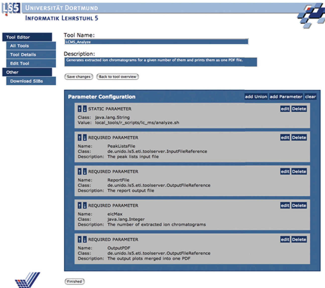
Figure 7 Defining the jETI SIBs within the HTML Configurator. This is the HTML Configurator of jETI used to specify a tool description. The picture shows the definition of the LCMS_Analyze Service specified as a command line call to a shell script with four required parameters taking two input files, a control value and one output file.
